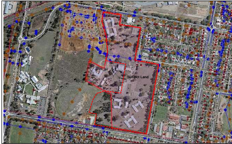
Figure 17: Sewer and Stormwater Assets Map (Source: WWCC 2021)
