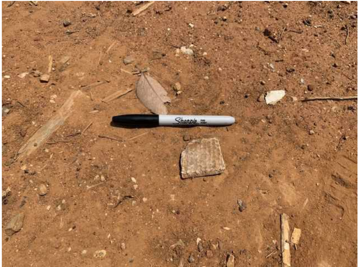
Photo 2. Typical surficial bonded asbestos material observed at the site.
