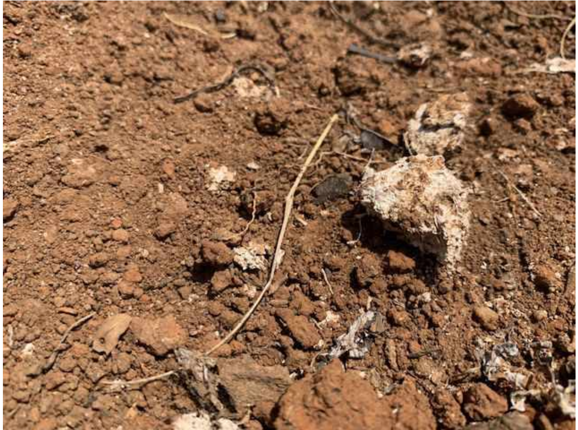
Photo 1. Fibrous lagging within Pit 347
