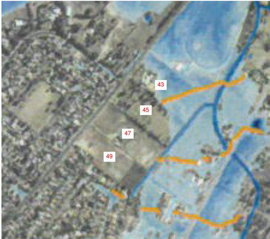
Figure 6: 2018 Overland Flow Flood Mapping, 1% AEP
